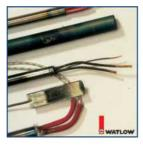
Tip 2: Protect leads and terminations from high temperatures and excessive movement Standard fiberglass-insulated lead wire may be used in applications with ambient temperatures up to approximately 260°C (500°F). If a lead is exposed to higher temperatures, high-temperature lead wire or ceramic bead insulation should be used. An unheated section of the heater, extending away from the heated region of the system, enables the leads to run at a beneficially cooler temperature.
